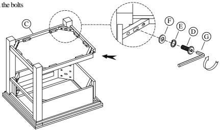
STEP 4: Using the Allen key (G) tighten all bolts
