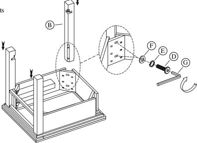
STEP 3: Do not fully tighten the bolts
